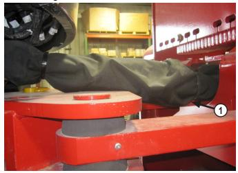
**2.** After routing the hoses through the undercarriage, route in the same location as the tractor's hoses (1). Replace zip ties if you run the hoses in the tractor's original hose cordura.
