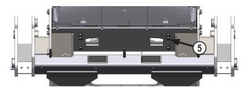
Note: If the tow cable bracket was equipped, reinstall the bracket when installing the front 6 vertical bolts. See Page 9 for more hardware and installation information.
