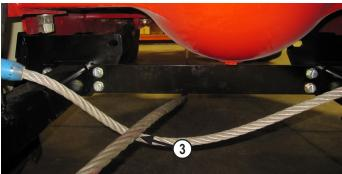
**3.** Route the cable underneath the undercarriage, then over the cable support and under the undercarriage on the right side (3).
