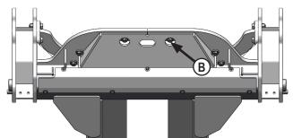
**6.** Lift the front of the undercarriage up and install 8 - 20mm x 90mm bolts and 8 - .375" thick washer from the bottom through the front slots of the undercarriage that line up with the vertical holes on the tractor frame **(B)**.
