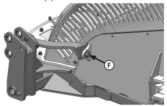
**15.** Attach the front upper support arms to the tractor with 2 - 1-1/4" x 4-1/2" bolt, 2 - 1-1/4" flat washer, and 2 - 1-1/4" nuts **(F)**.
