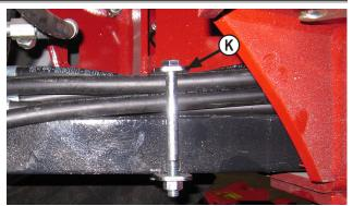
**6.** Strap the hoses to the drawbar with a set of hose holding plates in 2 locations **(K)**. Place 1 set as close to the front of the drawbar as possible and the other behind the axle before the hoses would be routed upwards to be plugged in.
