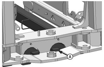
**5.** Lift the rear of the undercarriage up and set the top plates at the rear of the undercarriage on the tractor cross member **(A)**. Push the undercarriage back until the vertical push plates are firmly against the cross member.
