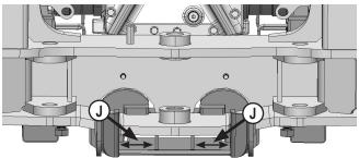
2. Send hoses through the bracket at the pivot point but stay on the outside of the rods that are by the center large nut on the tractor. The hoses should be between the rods and the inside plates of the bracket (J).
