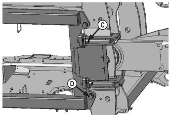
**8.** At the rear of the undercarriage and pivot area of the tractor, hook the rear hose routing bracket to the tractor frame and bolt to the rear of the undercarriage with 2- 1" x 3" bolts, 2 - 1" hardened washers, and 2. 1" nuts. The nut will fit between the plates on the
