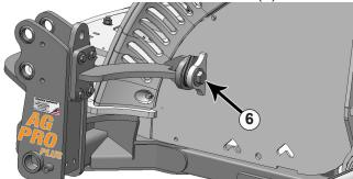
**16.** Attach the front upper support arms to the tractor with a 1-1/4" x 4-1/2" bolt and 1-1/4" flat washer on each side.
