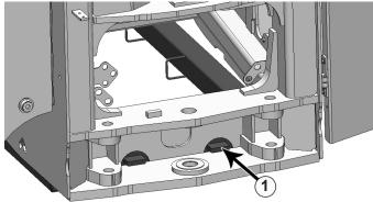
**5.** Lift the rear of the undercarriage and set the top plates on the tractor cross member (1). Push the undercarriage back until the vertical push plates are firmly against the cross member.
