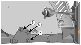
**17.** Install a side plate on each side of the undercarriage with 2 - 1" x 2" bolts and 2 - 1" ID x .375" thick washers (7).
