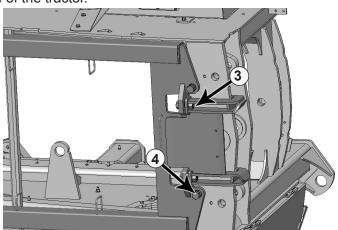
**10.** At the rear of the undercarriage and pivot area of the tractor, hook the rear hose routing bracket to the tractor frame and bolt to the rear of the undercarriage with  $1^{\circ} \times 3^{\circ}$  bolts,  $1^{\circ}$  hardened washers, and  $1^{\circ}$  nuts. The nut will fit between the plates on the brackets (3).
