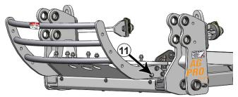
**26.** Install the grill guard to the front of the undercarriage with 3 - 3/4" x 1-3/4" bolts and 3 - 3/4" flat washers on each side (11).
