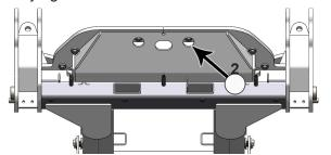
**6.** Lift the front of the undercarriage up and insert 6 - 1" x 3 - 1/2" bolts with a .375" thick washer on each bolt from the bottom through the front 6 slots of the undercarriage that line up with the vertical holes on the tractor frame (2). Hardware will be installed in remaining 2 slots in Step #8.
