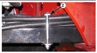
**6.** Strap the hoses to the drawbar with a set of hose holding plates in 2 locations (2). Place 1 set as close to the front of the drawbar as possible and the other behind the axle before the hoses would be routed upwards to be plugged in.
