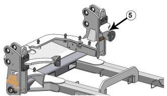
**15.** Attach the front upper support arms to the undercarriage with 4 - 3/4" x 2 - 1/2" bolts and 4 - 3/4" hardened flat washers on each side (5).
