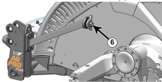
**14.** Attach the front upper support arms to the tractor with a 1-1/4" flat washer and 1-1/4" nut on each side (6).
