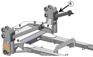
**13.** Attach the front upper support arms to the undercarriage with 4 - 3/4" x 2-1/2" bolts and 4 - 3/4" hardened flat washers on each side (5).
