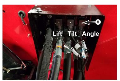
**33.** Guide the 3 cables and Dins from the wire harness out to the rear of the tractor.
