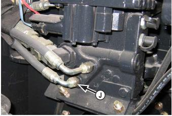
**15.** On the left side of the manifold valve, disconnect the bottom hydraulic line **(J)**.
