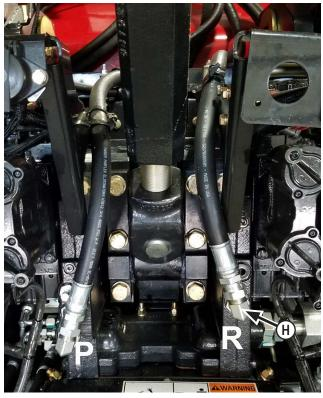
**NOTE:** Oil will flow. Be ready with an oil pan. **10.** Remove the plug or quick connect from the **P** and **R** ports at the rear of the tractor and replace each with a 90° fitting
