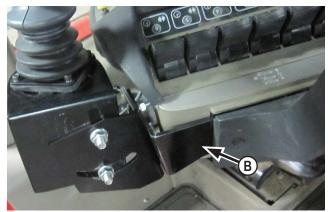
**2.** Attach the bolting plate (PN: 18-16713) along with the cover or monitor mount to the front of the armrest with the original hardware from step #1. Put the bracket between the armrest and the cover or monitor mount **(B)**.
