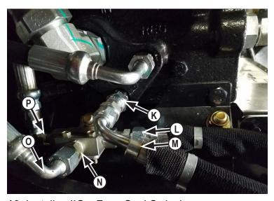
**16.** Install a JIC x Face Seal Swivel (PN: 31-12331-6-6) to the fitting that the hydraulic line was removed from **(K)**.
