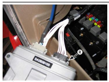
27. Set control box in fuse compartment (R).
