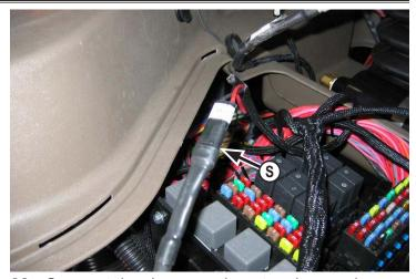
**28.** Connect the dozer angle extension cord (PN: 69-11663) to the wire harness **(S)**. Run the cord through the hole in the floor of the fuse compartment.
