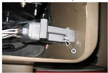
**38.** Drill a hole for a 1/4" bolt in the fuse compartment. Attach the wire harness to the compartment with a 1/4" bolt, 1/4" washer, and a 1/4" nut **(W)**.
