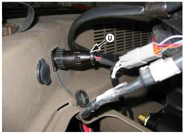
**32.** Plug the power cord from the wire harness into the port located behind and to the right of the operator's seat in the tractor cab **(U)**.
