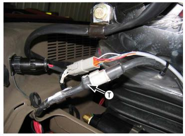
**31.** Connect the cable from the joystick to the wire harness **(T)**.
