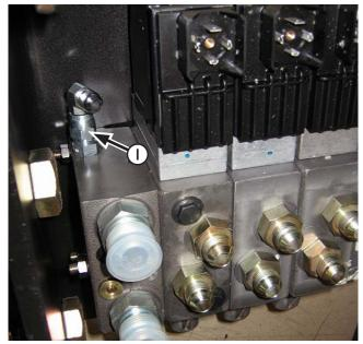
**13.** If fittings are not installed in the LS port on the control valve, install a straight -6-5 fitting (PN: 31-34033) and a 90° -6-6 fitting (PN: 31-34099) in the LS port (I).
