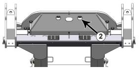
**6.** Lift the front of the undercarriage up and insert 8 - 20mm x 90mm bolts with a .375" thick washer on each bolt from the bottom through the front slots of the undercarriage that line up with the vertical holes on the tractor frame (2).
