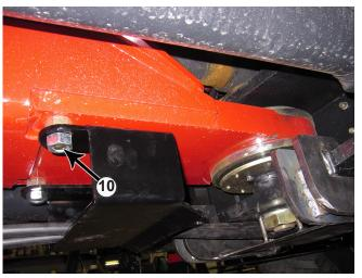
**22.** Attach the rear hose routing plate to the tractor frame behind the pivot point and before the drawbar. There will be 2 bolts sticking down. Attach with a 20mm nut on each side (10). Make sure the lip of the plate is facing towards the front of the tractor.
