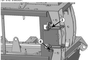
**8.** At the rear of the undercarriage and pivot area of the tractor, hook the rear hose routing bracket to the tractor frame and bolt to the rear of the undercarriage with  $1^{"} \times 3^{"}$  bolts,  $1^{"}$  hardened washers, and  $1^{"}$  nuts. The nut will fit between the plates on the brackets (3).
