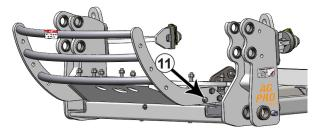
**24.** Install the grill guard to the front of the undercarriage with 3 - 3/4" x 1-3/4" bolts and 3 - 3/4" flat washers on each side (11).
