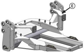
**14.** Attach the front upper support arms to the undercarriage with 2 - 1" x 3-1/4" bolts, 2 - 1" hardened flat washers, and a 1" nut on the top bolt on each side **(E)**.
