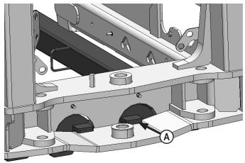
**5.** Lift the rear of the undercarriage up and set the top plates at the rear of the undercarriage on the tractor cross member **(A)**. Push the undercarriage back until the vertical push plates are firmly against the cross member.
