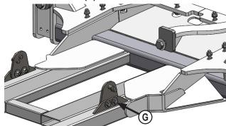
**16.** Install the front side tube bracket on each side of the undercarriage. The pins on the bracket will fit into the chain down hook on the inside of the tractor frame. Attach to the undercarriage with 2 - 3/4" x 2" bolts, 4 - 3/4" flat washers, and 2 - 3/4" lock nuts on each side **(G)**.
