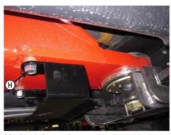
**20.** Attach the rear hose routing plate to the tractor frame behind the pivot point and before the drawbar. There will 2 bolts sticking down. Attach with 2 - 20mm nuts **(H)**. Make sure the lip of the plate is facing towards the front of the tractor.
