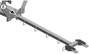
**8.** Position and center the push pole behind the undercarriage under the rear of the tractor. Lift and slide the font end of the push pole onto the round pin at the rear of the undercarriage **(E)**.
