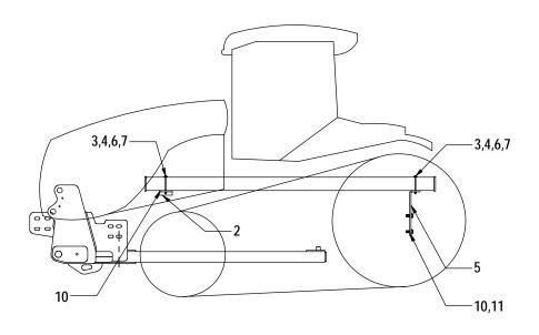
Note: Hose support bracket attached to tractor using front and rear step hardware.
