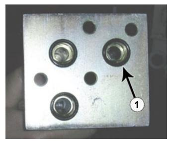
**10.** The back of the manifold cover (PN: 44-10247) with the three O-rings in place (1).
