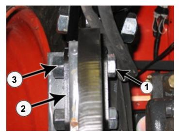
**26.** The heads of the bolts should be facing the inside of the tractor (1).
