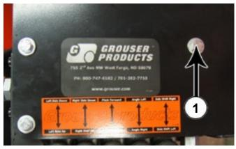
**36.** Attach the control valve (PN: 56-10280-B) to the valve stand with three 3/8" x 3/4" bolts (PN: 16-20062) and lock washers
