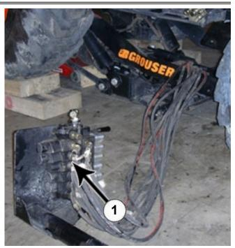
**20.** Guide the undercarriage and the valve stand under the tractor. Make sure that the valve and valve stand exit the right side of the tractor between the front and rear tires (1).
