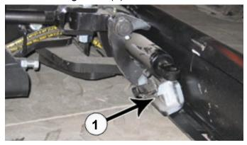
**52.** Lock the quick attach lever on each side (1). Verify that the lever engaged the corresponding slot on the bottom of the blade.
