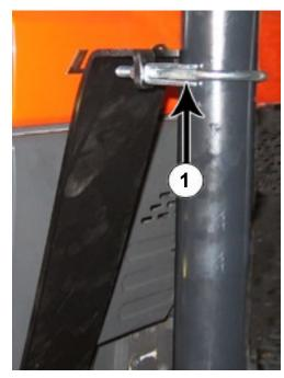
**34.** Attach the valve stand to the valve mount bracket with a U-bolt (PN: 16-10249) (1). Torque all bolts to the correct specification.
