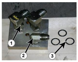
**9.** On the new manifold cover, install two straight fittings (PN: 31-34159) with a 90° fitting (PN: 31-34100) in the top two holes (1) and a 90° fitting (PN: 31-34170) in the bottom hole (2). Three O-rings (PN: 49-10246) (3) will be used on the back of the new manifold cover.
