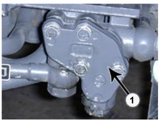
**11.** Remove the manifold cover and O-rings from the hydraulic supply manifold located under the operator's platform.
