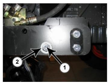
**28.** For the left and right undercarriage arms, insert a 5/8" x 2-1/2" bolt (PN: 16-20190) (1) with a 5/8" flat washer (PN: 57-20746) (2) into the final hole of the undercarriage arm along with a 5/8" flat washer and 5/8" center lock nut (PN: 70-20606) on the back side.
