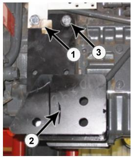
**16.** Remove and discard the right side hood bracket bolt, washer and spacer (1). The hood bracket will be reinstalled in the following step.
