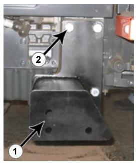
**14.** Install the left undercarriage bracket (PN: 18-10241) (1) with four 16mm x 1.50mm x 40mm bolts (PN: 16-1615040) (2).
