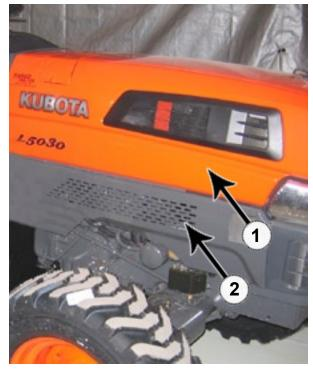
**8.** Lift the hood (1) of the tractor and remove the right side panel (2).
