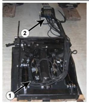
**19.** Align the undercarriage (1) behind the tractor. Lay out the valve and hoses in front of the undercarriage (2). The hoses should be over the right undercarriage arm.
