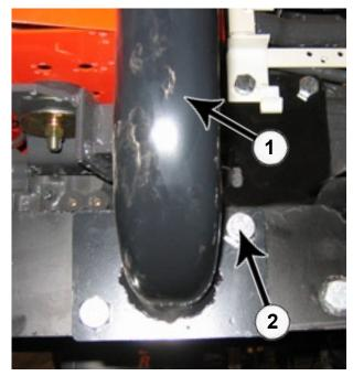
**33.** Align the valve stand (PN: 17-10235) (1) with the undercarriage. Use two 3/4" x 2" bolts (PN: 16-20218) (2) with two 3/4" center lock nuts (PN: 70-20607) to securely attach the stand to the undercarriage.
