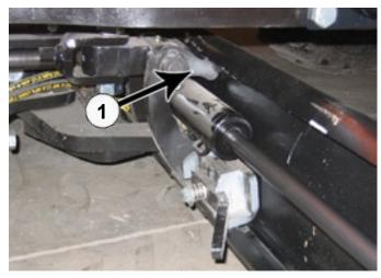
**51.** Pitch the male quick attach back to lift the blade off the ground (1).
