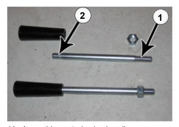
**41.** Assemble control valve handles (PN: 39-10199). Put the nut on the side of the bolt that has longer threads (1). Put the black handle on the other end that has shorter threads (2).
