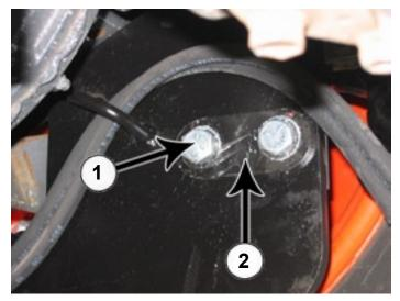
**25.** For the left and right side, insert two 5/8" x 2-1/2" bolts (1) (PN: 16-20190) with a 2 hole washer (2) (PN: 57-11452).
