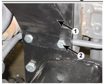
**32.** Attach valve mount bracket (PN: 18-10238) (1) to the right undercarriage bracket with two 1/2" x 1-1/2" bolts (PN: 16-20126) (2) and two 1/2" center lock nuts (PN: 70-20604).
