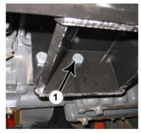
**15.** One lower bolt is inside the mounting bracket (1).
