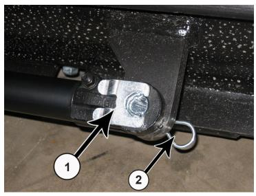
**58.** Extend the side shift cylinder out to the cylinder connector. Insert pin (PN: 43-7995) (1) and the clip pin (PN: 43-7767) on the bottom (2).
