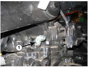
**24.** Remove Tank plug and install the 45° fitting (PN: 31-34183) into the Tank port located behind and above the right axle (1).
