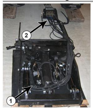
**26.** Align the undercarriage (1) behind the tractor. Lay out the valve and hoses in front of the undercarriage (2).
