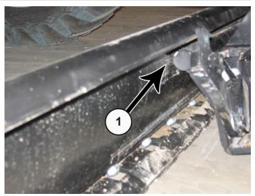
**55.** Pitch the male quick attach forward. Position the blade so the top round bar will hook under blade lip (1).
