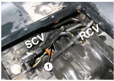
**20.** Locate and remove the SCV to RCV hydraulic oil line below and to the right of the seat area (1).
