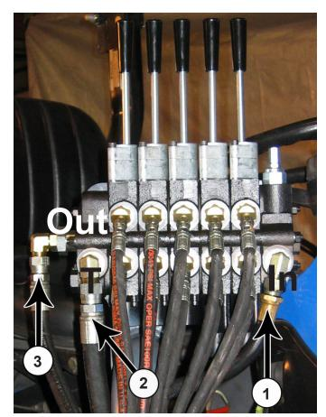
**46.** Attach the previously installed 101" hose from Step #21 to the **In** port on the BBCV (1).
