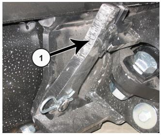
**57.** Lock the quick attach lever on each side (1). Verify that the lever engaged the corresponding slot on the bottom of the blade.
