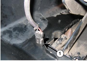
**19.** Remove seat and disconnect the seat safety connector (1).
