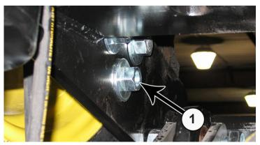
**32.** Secure the undercarriage to the rear brackets by installing a 3/4" flat washer (PN: 57-20747) and 3/4" nut (PN: 70-20607) on each bolt that was installed in the previous step (1).
