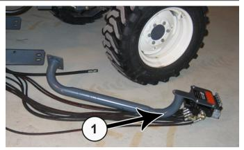
**27.** Guide the undercarriage and the valve stand under the tractor. Make sure the valve and valve stand exit the right side of the tractor (1).
