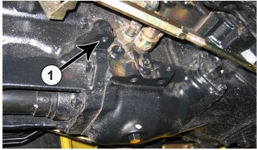
**30.** Attach the middle of the undercarriage to the tractor above the drive shaft and in front of the oil drain with a  $12\text{mm} \times 40\text{mm}$  bolt (PN: 16-1217540) and a 7/16" washer (PN: 57-20743) on each side (1).
