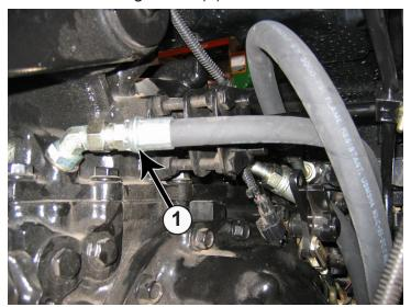
**25.** Attach the 90" hose (PN: 35-30039) to the 45° fitting from the previous step (1). Route the hose to the front right side of the operator platform and lay the end of the hose on the platform. The hose will be attached later to the BBCV in Step #47.
