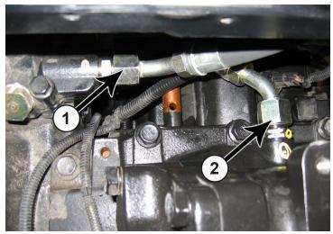
**21.** Attach the 101" hose (PN: 35-10226) to the SCV side of the tractor transmission (front fitting) (1).
