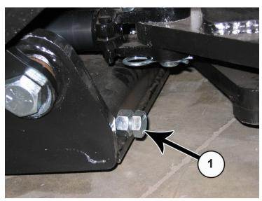
**61.** Adjust angle stops (1) so blade does not interfere with tires during angle of blade. Use a wrench to loosen the nut and to the turn the bolt either in or out depending if the blade is hitting the tire. After adjustment, tighten the nut.
