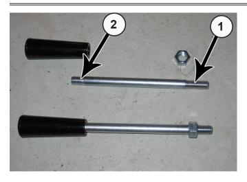
**43.** Assemble control valve handles (PN: 39-10199). Put the nut on the side of the bolt that has longer threads (1). Put the black handle on the other end that has shorter threads (2).
