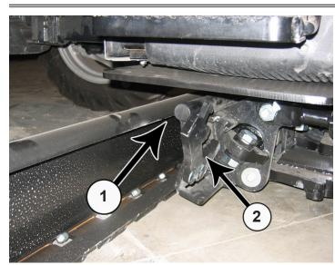
**54.** Slide blade under tractor until the quick attach is in line with the center of the blade (1). Make sure that the quick attach locking levers are still up (2).
