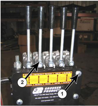
**44.** Attach the control valve to the valve stand with 3 - 3/8" x 3/4" bolts (PN: 16-20062) and 3 - 3/8" lock washers (PN: 57-20762) (1).
