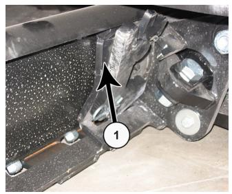
**56.** Pitch the male quick attach back to lift the blade off the ground (1).
