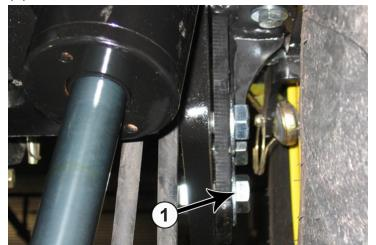
**31.** Continue to raise the rear of the undercarriage between the rear brackets until the rear holes line up with the holes on the rear brackets. Insert 3 - 3/4" x 2-1/4" bolts (PN: 16-20219) with a 3/4" flat washer (PN: 57-20747) on each bolt through the holes of the bracket and undercarriage on both sides (1).
