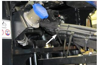
1. Route the hoses from the bulkhead fittings at the middle of the undercarriage thru all the hose loops on the undercarriage. Once at the end of the undercarriage route the hoses up along the tractor frame following any of the tractor's hoses while still staying away from any sharp corners and moving parts.
