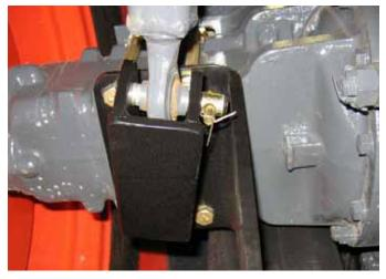
**11.** Attach the 3-point hitch to the new bracket with the origal hardware.
