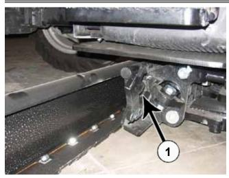
**43.** Slide blade under tractor until the quick attach is approximately in the center of the blade. Make sure that the quick attach locking levers are still open (1).
