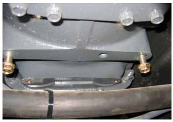
**14.** Remove fuel tank cross protection tube from under the tractor.
