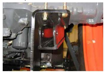
**10.** Attach the rear brackets (PN: 14425-R,L) to the rear axle with the original hardware the same way as the originals were attached. Verify that the 3-point hitch connection is pointing in the correct direction.
