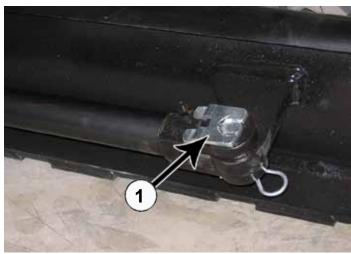
**47.** Extend the side shift cylinder out to the cylinder connector. Insert pin (PN: 43-7995) and the clip pin (PN: 43-7767) on the bottom (1).
