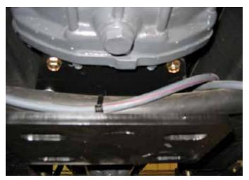
**15.** Install the center bracket (PN: 18-10539) so the open section faces the rear and the fuel tank hoses are protected in the bracket. Use 12mm x 25mm bolts (PN: 16-1212525) and a 12mm washer (PN: 57-20823) in the rear holes and 12mm x 35mm bolts (PN: 16-1212535) and a 12mm washer (PN: 57-20823) in the front holes.
