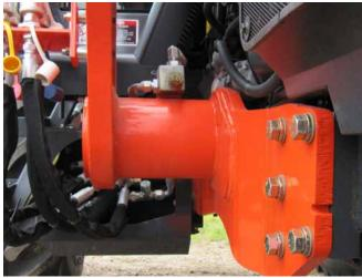
**36.** Attach 98" hose (PN: 35-111689-0980) from the Out Port on the electric valve to the In port on the loader valve that the hose was removed from.
