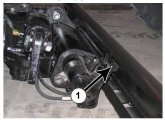
**44.** Pitch the male quick attach forward. Position the blade so the top round bar will hook under blade lip (1).
