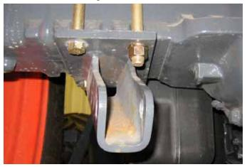
**9.** Remove nut and washer from rear bolt on the 3-point hitch bracket on rear axle. Remove remaining 3 bolts, washers, and nuts along with the 3-point hitch bracket.
