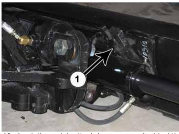
**46.** Lock the quick attach lever on each side (1). Verify that the lever engaged the corresponding slot on the bottom of the blade.
