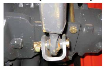
**8.** Remove 3-point hitch from rear axle bracket from the left and right side.
