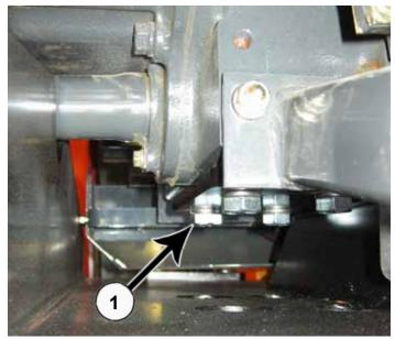
**35.** Attach the front of the undercarriage to the tractor with four 16mm x 40mm bolts (PN: 16-1615040) with a 16mm lock washer (PN: 57-20834) on each bolt (1).
