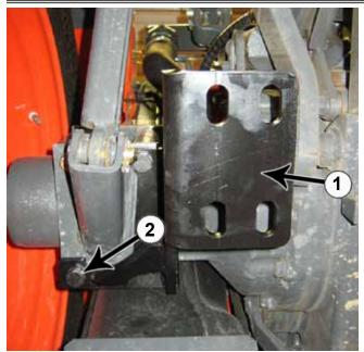
**27.** Remove three bolts from the 3-point hitch brace from the bottom of the left rear axle. Attach left rear bracket (PN: 18-11735-L) (1) with three 16mm x 50mm bolts (PN: 16-1615050) and a 16mm lock washer (PN: 57-20835) on each bolt (2).
