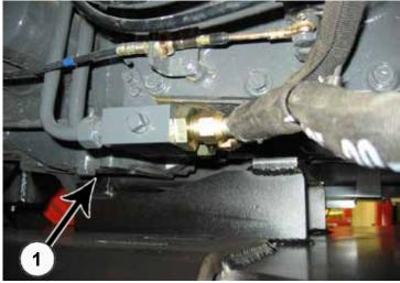
**33.** Raise the undercarriage up to the installed tractor brackets and the tractor frame. The bolts are already in the brackets. Line up the undercarriage so all bolts go through their corresponding holes on the undercarriage and the holes on the undercarriage line up with the holes in the tractor frame (1).
