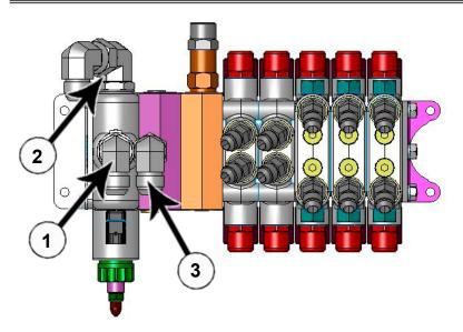
**22.** If hydraulic fittings are not installed, install a 90° fitting (PN: 31-34054) in the **In** (1) and **Out** (2) Ports on the electric valve.
