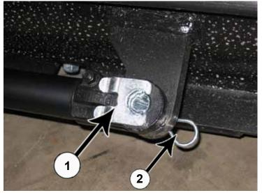
**52.** Extend the side shift cylinder out to the cylinder connector. Insert pin (PN: 43-7995) (1) and the clip pin (PN: 43-7767) on the bottom (2).
