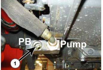
**10.** Remove plugs (1) from the outlet block located under the operator platform and replace with 2 - #12 fittings (PN: 31-11741) including the bonded seal.
