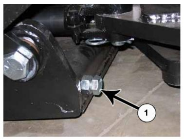
**55.** Adjust angle stops (1) so blade does not interfere with tires during angle of blade. Use a wrench to loosen the nut and to the turn the bolt either in or out depending if the blade is hitting the tire. After adjustment, tighten the nut.
