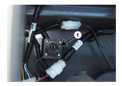
20. Attach the power cord from the valve controller to the auxiliary power socket (1).21. Run the wire harness to the electric valve. Connect the colored wires from the wire harness to their corresponding port on the back of the electric valve. Refer to the diagram on Page 13-14.
