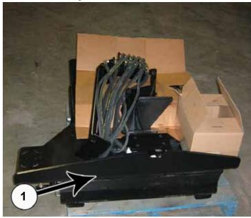
**5.** The Belly Blade will arrive on a pallet. Unwrap and set the blade aside. Remove the undercarriage assembly from the pallet (1).
