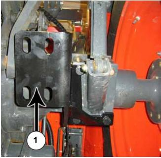
28. Repeat Step #27 for the right side with the right rear bracket (PN: 18-11735-R) (1).Note: Verify the correct orientation of the rear brackets.
