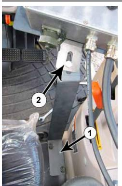
**14.** Attach the brace plate (PN: 44-14443) to the platform on the right side of the seat (1). Use the original hardware.
