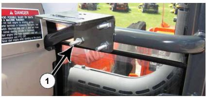
**15.** Attach the connecting plate (PN: 44-14448) to the handle by the front right window (1). Use 2 - u-bolts.
