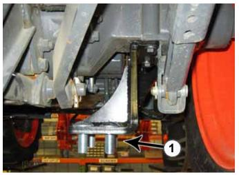
**32.** Insert four 3/4" x 2" carriage bolts (PN: 16-21218) into the installed rear right bracket (1). These should be inserted from the top and will be used to attach the undercarriage.
