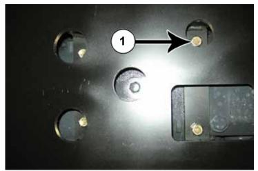
**34.** Use four 14mm x 40mm bolts (PN: 16-1415040) with a 14mm lock washer (PN: 57-20834) on each bolt to attach the middle of the undercarriage to the tractor (1).
