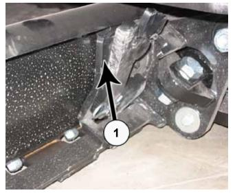
**50.** Pitch the male quick attach back to lift the blade off the ground (1).
