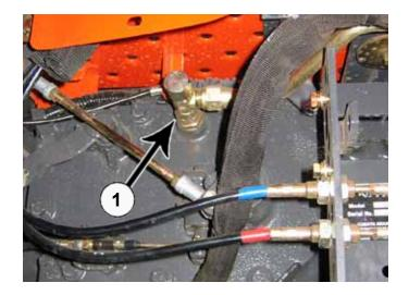
**12.** Remove plug from the Tank Port located under the operator platform and replace with a #8 fitting (PN: 31-11740) including the bonded seal (1).
