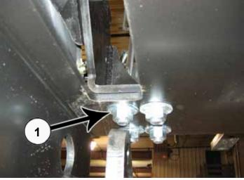
**36.** Use eight 3/4" flat washers (PN: 57-20747) and 3/4" center lock nuts (PN: 70-20607) to attach the undercarriage to the rear brackets (1).
