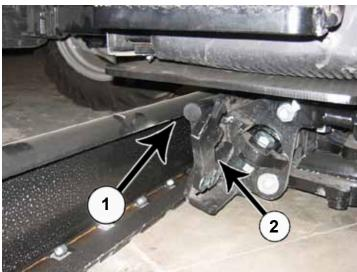
**48.** Slide blade under tractor until the quick attach is in line with the center of the blade (1). Make sure that the quick attach locking levers are still up (2)
