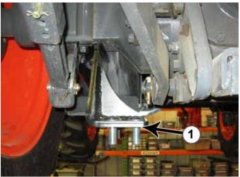
**31.** Insert four 3/4" x 2" carriage bolts (PN: 16-21218) into the installed rear left bracket (1). These should be inserted from the top and will be used to attach the undercarriage.
