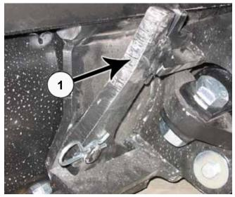
**51.** Lock the quick attach lever on each side (1). Verify that the lever engaged the corresponding slot on the bottom of the blade.
