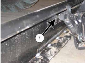
**49.** Pitch the male quick attach forward. Position the blade so the top round bar will hook under blade lip (1).
