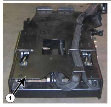
**29.** Align the undercarriage (1) behind the tractor.
