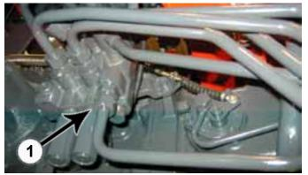
**14.** Remove fitting and hydraulic line from the tank port on the loader control valve (1). Plug the end of the hydraulic line. The other end of the hydraulic line will be removed in Step #17.
