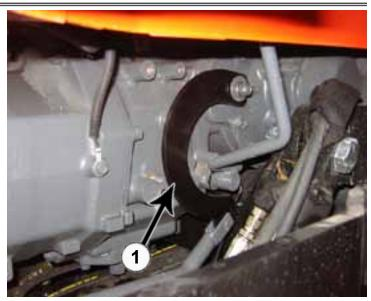
**13.** Remove the left brake lever and replace with new brake lever (PN: 11-11782) (1).
