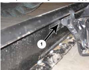
**47.** Pitch the male quick attach forward. Position the blade so the top round bar will hook under blade lip (1).
