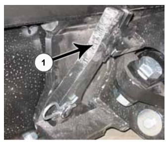
**49.** Lock the quick attach lever on each side (1). Verify that the lever engaged the corresponding slot on the bottom of the blade.
