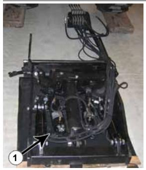
**22.** Align the undercarriage (1) behind the tractor. The hoses should be over the right undercarriage arm.
