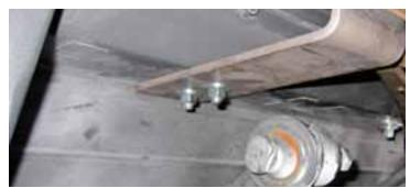
**35.** Remove the slow moving vehicle sign and bracket. Attach the valve bracket to the rear of the tractor where the sign bracket was attached and drill 2 more holes next to the original set. Use the bracket as a guide. The left side of the bracket will go on the outside of the tube frame. You'll need to drill holes and attach to these tubes or weld the bracket to the frame if you prefer to do that.
