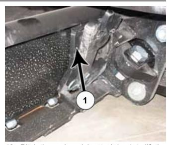
**48.** Pitch the male quick attach back to lift the blade off the ground (1).
