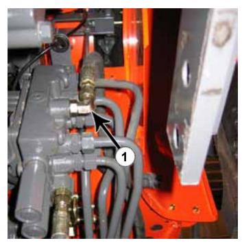
**19.** Remove fitting and hydraulic line from the Power Beyond port on the loader control valve. Replace with a 90° fitting (PN: 31-34050), a bonded seal (PN: 49-11801-20), and a 53" hose (1). Lay the other end of the hose on the operator's platform. The hose will be attached later to the electric valve in Step #38.
