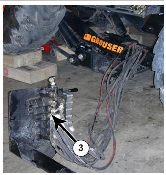
**14.** Guide the undercarriage and the valve stand under the tractor. Make sure that the valve and valve stand exit the right side of the tractor between the front and rear tires (3).
