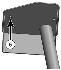
**28.** Attach the control valve (PN: 56-10200) to the valve stand with three 3/8" x 3/4" bolts (PN: 16-20062) and lock washers (PN: 57-20762) (5).
