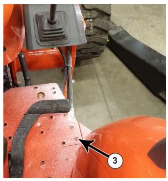
**NOTE:** Photo to show where the valve mount support will be installed (3).
