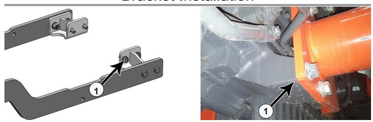
**15.** Install the front brackets to the front side of the tractor where the loader mounts are attached with 2 - 16mm x 40mm bolts (PN: 16-1615040) and a 5/8" flat washer (PN: 57-20756) on each bolt on each side (1). Picture on the right shows a loader bracket and is used to only show where the front brackets get mounted.
