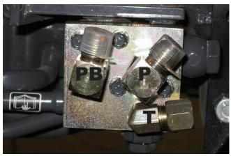
**12.** Attach a 57" hose to the PB and the T ports. Attach a 54" hose to the P port. Lay the other ends of the hoses on the operator's platform to keep them out of the way for installing the undercarriage. The hoses will be attached later in Steps #31-33.
