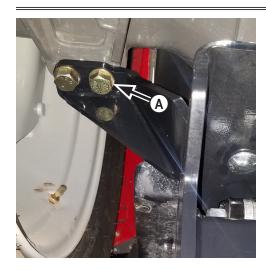
**8.** Remove front two bolts from 3-point hitch brace on right and left rear axle. Attach rear brackets with 2 - 20mm x 150mm bolts and 2 - 3/4" flat washers (A).
