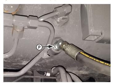
**28.** Remove plug from tank below the operator station. Install a 45° fitting and attach opposite end of 72" hose from Tank port on Belly Control Valve from Step #26 **(P)**.
