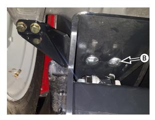
**11.** Use 4 - 3/4" x 2" carriage bolts, 4 - 3/4" flat washers and 4 - 3/4"nuts **(B)** to attach rear brackets to undercarriage.
