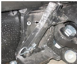
**40.** Lock the quick attach lever on each side **(Y)**. Verify that the lever engaged the corresponding slot on the bottom of the blade.
