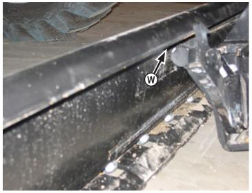
**38.** Pitch the male quick attach forward. Position the blade so the top round bar will hook under blade lip **(W)**.
