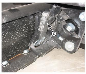
**39.** Pitch the male quick attach back to lift the blade off the ground **(X)**.
