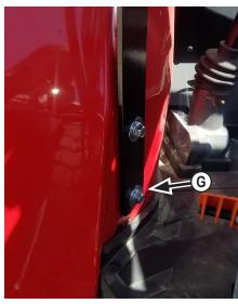
**16.** Attach the valve support plate to the front of the right fender with 2 - 3/8" x 1" flange bolts, 4 - 3/8" fender washers and 2 - 3/8" nyloc nuts **(G)**.6
