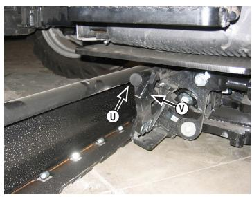
**37.** Slide blade under tractor until the quick attach is in line with the center of the blade **(U)**. Make sure that the quick attach locking levers are still up **(V)**.
