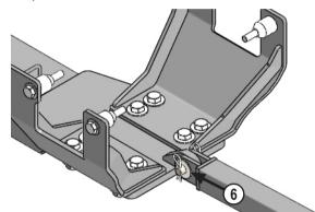
**15.** Attach the front of the push pole to the rear of the undercarriage with a pin, 2 - 1" washers, and 2 - pin clips **(6)**.
