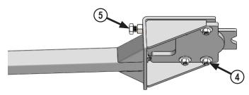
**12.** Attach the push plate to the rear of the push pole with 4 - 3/4" flat washers and 4 - 3/4" nuts **(4)**. The round edge of the push plate should be towards the open back of the push pole.
