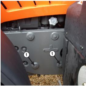
**2.** If tractor doesn't have loader brackets, remove the bottom 2 plugs from the holes on each side of the tractor behind the front tires **(1)**.
