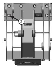
**8.** Attach the front of the undercarriage to the front of the tractor nose casting with 6 - 20mm x 70mm and 6 - 3/4" hardened flat washers **(2)**.
