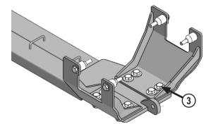
**9.** Attach the rear of the undercarriage to the side rails with 4 - 1" bolts, 8 - 1" flat washers, and 4 - 1" nuts on each side **(3)**.
