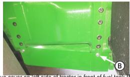
Remove cover on left side of tractor in front of fuel tank (B).
