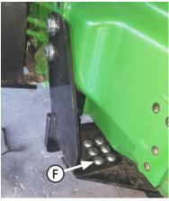
**10.** Attach rear brackets to rear of undercarriage with 12 - 3/4" x 2" carriage bolts, 12 - 3/4" flat washers and 12 - 3/4" center lock nuts **(F)**.
