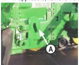
2. If applicable, remove implement quick coupler and bracket from right side of tractor (A).
