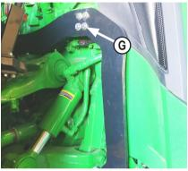
**11.** Attach side rails to side of tractor with 12 - 16mm x 90mm bolts and 12 - 5/8" flat washers **(G)**.
