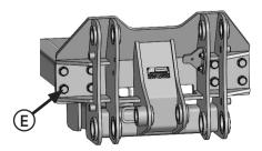
9. Attach front of undercarriage to tractor with 8 - 20mm x 70mm bolts and 8 - 3/4" flat washers (E).
