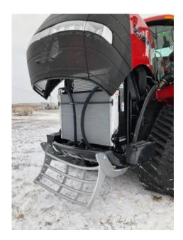
Rotates Down for Access to Hood Latch and Coolers. For use with Scraper Tractors or standard Ag Tractors wanting front grille protection.
