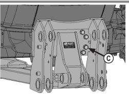
Attach front of undercarriage to front of tractor with 8 - 20mm x 70mm bolts and 8 - 3/4" hardened flat washers (C).
