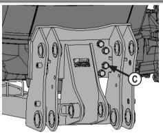
Attach front of undercarriage to front of tractor with 8 - 20mm x 70mm bolts and 8 - 3/4" hardened flat washers (C).
