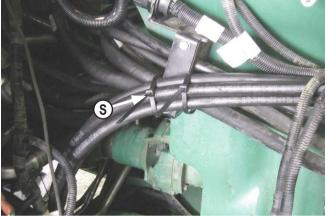
Route hoses upward through tractor. Staying away from the driveshaft by attaching hoses to any other steel lines along way. Attach to tractor's hoses right by hose bracket with zip ties (S).
