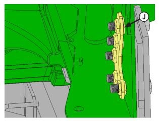
Thread a 3/4" flange nut on top 4 bolts from Step #17. Attach nut plate to bottom bolt and line up top hex nuts to fit in nut plate (J). Note orientation of flange nuts.
