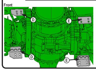
Loosely attach front brackets to front 3 holes on tractor frame in front of axle with 6 - 24mm x 50mm bolts and 6 - 7/8" hardened washers (D). Note orientation of the brackets.
