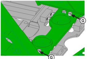
14. Attach rear of undercarriage vertically to cross member on tractor frame behind front axle with 4 - 7/8" x 3" bolts, 8 - 7/8" hardened flat washers, and 4 - 7/8" nuts (G).
