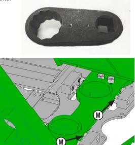
25. Unscrew 1" x 2" bolts (M) at rear of undercarriage until they are tight against tractor frame. Torque 1" bolts to 200 ft-lbs.
