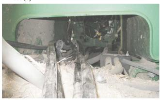
6. Route hoses through open cavity of back section of tractor. Secure hoses with zip ties where necessary to avoid rubbing and pinch areas. Plug hoses into open SCV's at back of tractor.
