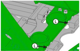
22. Unscrew 1" x 2" bolts (L) at rear of undercarriage until they are tight against tractor frame. Torque 1" bolts to 200 ft-lbs.
