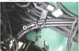
Route hoses upward through tractor. Staying away from driveshaft by attaching hoses to any other steel lines along way. Attach to tractor's hoses right by hose bracket with zip ties (R).
