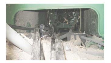
6. Route hoses through open cavity of back section of tractor. Secure hoses with zip ties where necessary to avoid rubbing and pinch areas. Plug hoses into open SCV's at back of tractor.
