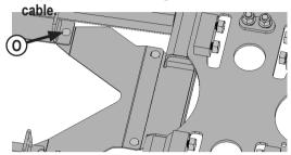
26. Install hose guard plate to rear of undercarriage with 4 - 1/2" x 1" carriage bolts, 4 - 1/2" washers and 4 - 1/2" nuts
