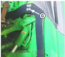
Attach side rails to side of tractor with 12 - 16mm x 90mm bolts and 12 - 5/8" flat washers (G).
