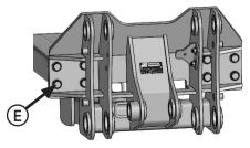
9. Attach front of undercarriage to tractor with 8 - 20mm x 70mm bolts and 8 - 3/4" flat washers (E).
