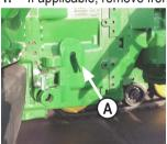
If applicable, remove implement quick coupler and bracket 2. from right side of tractor (A).
