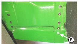
3. Remove cover on left side of tractor in front of fuel tank (B).
