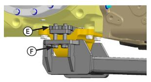
8. Place clamp weld bracket on top of drawbar bracket (E).
