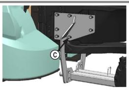
Attach side brackets to tractor with 14 - 20mm x 50mm bolts and 14 - 3/4" flat washers (C).
