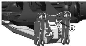
4. Lift undercarriage and attach front of undercarriage to tractor with 8 - 20mm x 70mm bolts and 8 - 3/4" flat washers (B).
