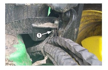
7. Secure hoses with a velcro strap (T) above rear axle with original hardware.
