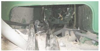
6. Route hoses through open cavity of back section of tractor. Secure hoses with zip ties where necessary to avoid rubbing and pinch areas. Plug hoses into open SCV's at back of tractor.
