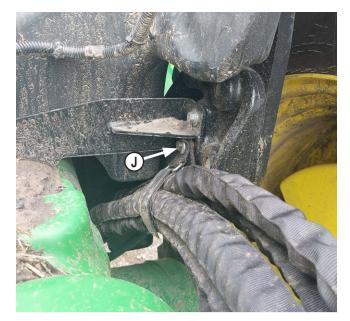
Secure hoses with a velcro strap (J) above rear axle with original hardware.
