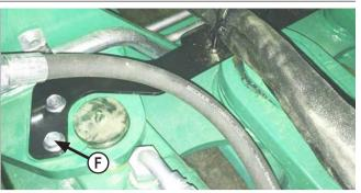
5. At pivot area of tractor, remove bolts from top plate that hold the cylinder pins and install hose routing bracket along with original plate and new 12mm flange bolts. Verify front leg of bracket is formed down. Torque 12mm bolts to 105 ft-lbs (F).
