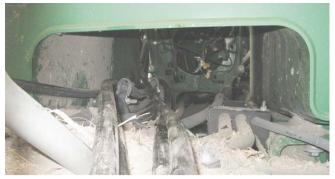
Route hoses through open cavity of back section of tractor.
