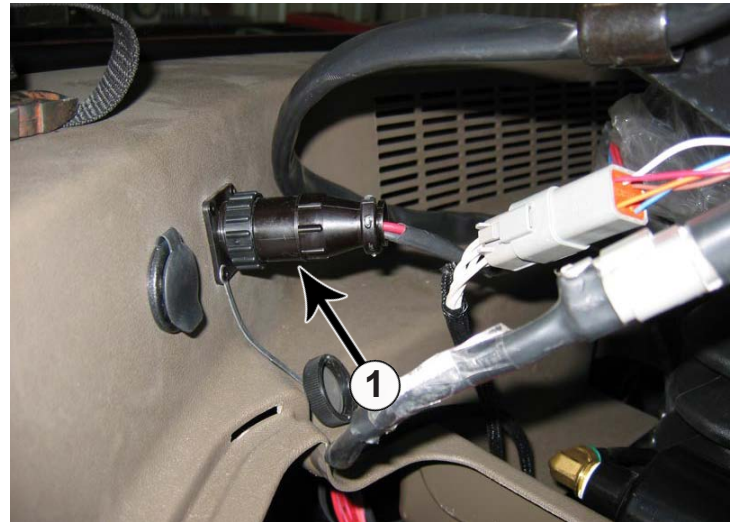
26. Plug the power cord from the wire harness into the port located behind and to the right of the operator's seat in the tractor cab (1).
