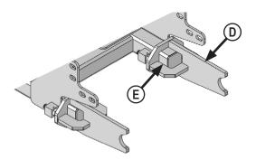
5. Install the rear brackets on the rear undercarriage. The orientation of the bracket should be as shown in the photo. The flat edge of the plate should be on the top (D) and the larger opening for the tube on the inside (E).
