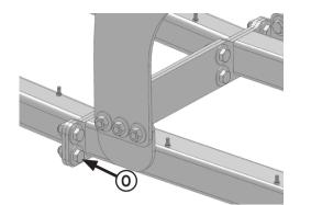
**17.** Attach the front undercarriage to the rear undercarriage with  $8 - 7/8^{\circ} \times 2 - 1/2^{\circ}$  bolts,  $16 - 7/8^{\circ}$  flat washers, and  $8 - 7/8^{\circ}$  nuts (**O**).
