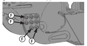
6. In front of the rear axle, remove the front 2 bolts and bottom 2 bolts on each side (F). The washers will be reused in Step #8.
