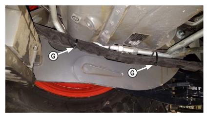
**5.** Route the hoses and secure with hose straps along the undercarriage until you reach the end of the undercarriage.
