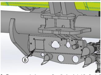
**3.** Remove any wire harnesses from the bracket at the front of the tractor and remove the front bracket **(B)**. Wire harnessess will be reattached to the undercarriage.
