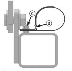
Attach a velcro hose strap on every bolt along rear undercarriage with a 3/8" flange nyloc nut (C). Assemble strap with the metal loop on top side as shown (D). Keep straps open.
