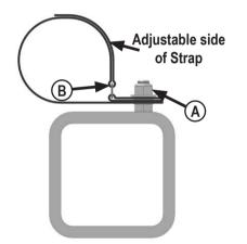
1. Attach a velcro hose strap on every bolt along front undercarriage with a 3/8" flange nyloc nut (A). Assemble strap with the metal loop on top side as shown (B). Keep straps open.
