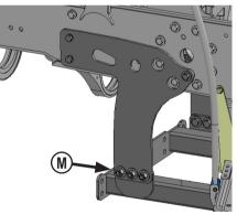
14. Attach the side plates to the rear undercarriage with 6 - 7/8" x 2-1/4" bolts, 12 - 7/8" flat washers, and 6 - 7/8" nuts (M).
