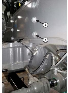
**2.** Behind the front axle, remove the bottom 2 bolts from each side of the tractor. You will reuse the washers in Step # 10 (A).
