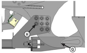
**7.** Position the rear undercarriage under tractor and center on the frame of the tractor.
