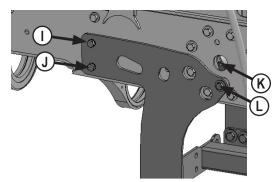
**10.** Attach the side plate to the tractor frame with 2 - 20mm x 130mm bolts and 2 - orignal tractor 20mm washers in the front top hole **(I)**.
