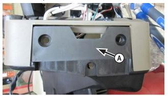
**1.** Remove the cover or the monitor mount from the front of the armrest **(A)**.
