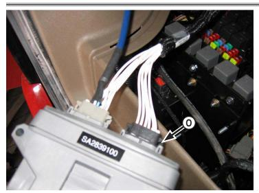
26. Set control box in fuse compartment (O).
