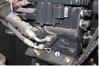
**16.** On the left side of the manifold valve, disconnect the bottom hydraulic line **(J)**.
