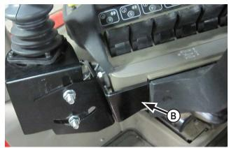
**2.** Attach the bolting plate (PN: 44-16713) along with the cover or monitor mount to the front of the armrest with the original hardware from step #1. Put the bracket between the armrest and the cover or monitor mount **(B)**.
