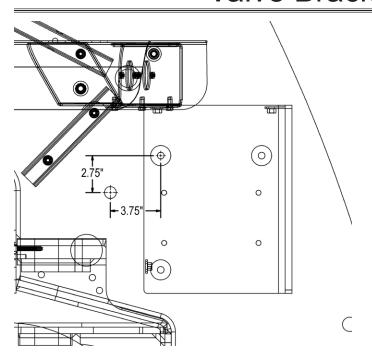
**7.** Drill the first 1/2" hole for the rear valve mount below the rear left fender. After first hole is drilled, use the valve mount as a guide to mark other 2 holes. Drill remaining 2 holes for valve mount.
