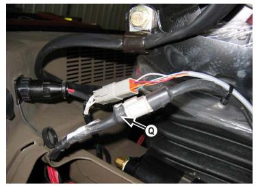
**27.** Connect the cable from the joystick to the wire harness **(Q)**.
