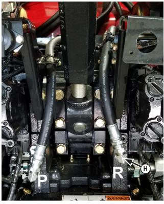
**NOTE:** Oil will flow. Be ready with an oil pan. **11.** Remove the plug or quick connect from the **P** and **R** ports at the rear of the tractor and replace each with a 90° fitting (PN: 31-34259) **(H)**.
