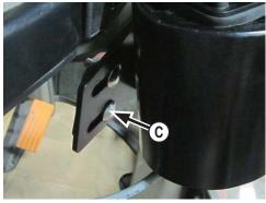
**3.** Attach the small middle bolting plate (PN: 44-16712) to the bracket from Step #2 with 2 - 3/8" x 1" carriage bolts and 2 - 3/8" flange nuts **(C)**.
