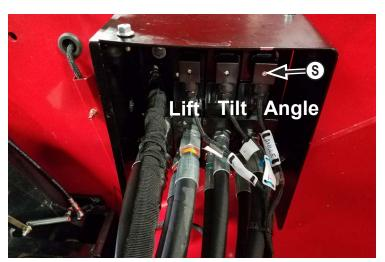
**29.** Guide the 3 cables and Dins from the wire harness out to the rear of the tractor.
