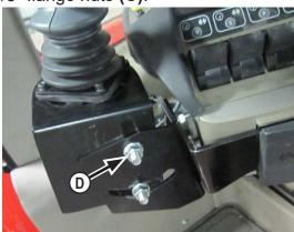
**4.** Attach the joystick mount (PN: 18-16705) to the bracket from Step #3 with 2 - 3/8" x 1" carriage bolts and 2 - 3/8" flange nuts **(D)**.
