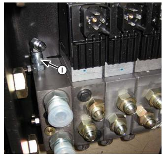
**14.** If fittings are not installed in LS port on control valve, install a straight -6-5 fitting (PN: 31-34033) and a 90° -6-6 fitting (PN: 31-34099) in LS port (I).
