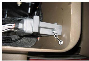
**34.** Drill a hole for a 1/4" bolt in the fuse compartment. Attach the wire harness to the compartment with a 1/4" bolt, 1/4" washer, and a 1/4" nut **(T)**.
