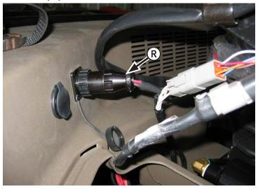
**28.** Plug the power cord from the wire harness into the port located behind and to the right of the operator's seat in the tractor cab **(R)**.
