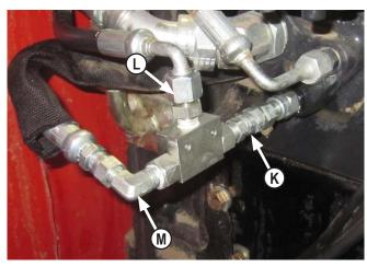
**17.** Install a JIC x Face Seal Swivel (PN: 31-12331-6-6) to the fitting that the hydraulic line was removed from. Also install a Female JIC Swivel x Male Pipe fitting (PN: 31-12332-6-4) onto the previous fitting
