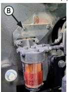
For 8700 S tractors - Remove fuel filter on left side and flip bracket upside down (B). Reinstall fuel filter.
