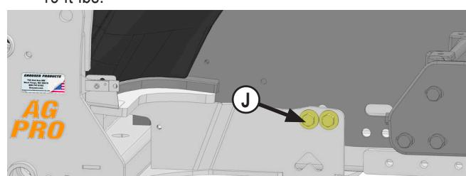
15. Attach side plate of undercarriage to tractor with 4 - 7/8" x 2-1/2" bolts, 8 - 7/8" washers, and 4 - 7/8" nuts in tie down hook holes (J).
