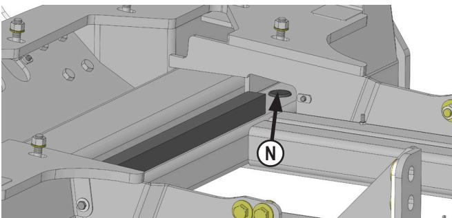
24. Install 2 ribbed plugs in holes on top of undercarriage tube (N).
