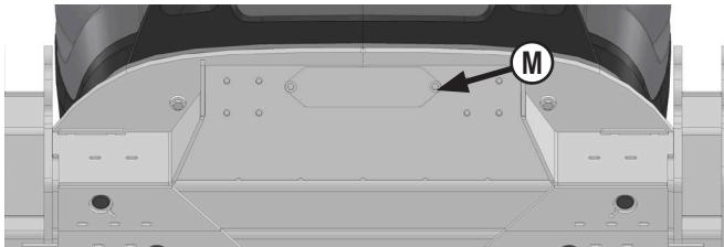
20. Attach front cover plate to undercarriage with 2 - 1 1/2" x 1-1/4" bolts and 2 - 1 1/2" washers (M).
