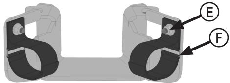
5. Secure hose straps to bottom cover plate with 3/8" x 1" carriage bolts and 3/8" flange nyloc nuts (E). Attach strap with metal loop on bottom side of strap (F). Keep straps open until securing hoses.
