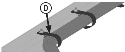
4. Route hoses along undercarriage tubes and secure with velcro straps (D).
