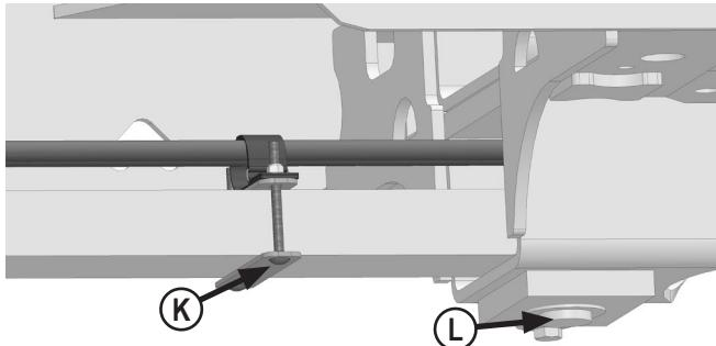
11. Install front holding plates (K) 12" from center of drawbar pin at front of drawbar (L) with 2 - 3/8" x 4-1/2" carriage bolts, 1 or 2 hose straps and 2 - 3/8" flange nuts.
