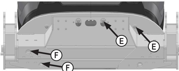
9. At front of undercarriage, install 4 - 20mm x 90mm bolts, 4 - 3/4" ID x .375" thick washers, 4 - 3/4" flat washers and 4 - 20mm nuts in front vertical slots (E).
