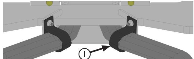
8. Continue routing hoses through cover plate. Secure hoses with velcro straps (I).
