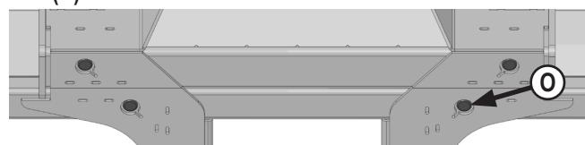
25. Install 4 ribbed plugs in holes on bottom of undercarriage (O).
