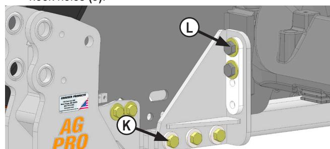
16. Remove 27mm bolts and spacers from front axle on both sides of tractor. Discard spacers.
