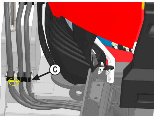
2. Route hoses behind boxbeam of undercarriage. Lift hoses in outer clamp. Angle and tilt hoses on inner clamps. See tractor hydraulics page in lift system parts book for correct hose clamp and hardware.
