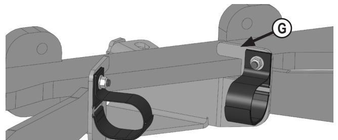
6. Lift bottom cover plate into place with hoses between cover plate and bottom of undercarriage. Set cover plate on rear cross member of undercarriage (G).
