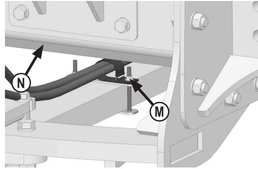
13. Install rear holding plates (M) half-way between rear axle and rear tractor frame (N) with 2 - 3/8" x 4-1/2" carriage bolts, 1 or 2 hose straps and 2 - 3/8" flange nuts.
