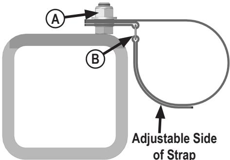
1. Attach a velcro hose strap on every bolt along undercarriage with a 3/8" flange nyloc nut (A). Assemble strap with the metal loop on bottom side as shown (B). Keep straps open.
