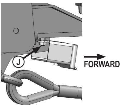
9. Gather and position hoses inside hose routing bracket. Raise rear hose routing bracket with hoses and attach to 20mm bolts located at front of rear tractor frame behind pivot area. Attach with 2 - 20mm nuts (J). Ensure lip of bracket is facing towards front of tractor.
