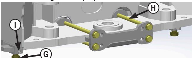
11. Tighten rear vertical bolts evenly (G) to pull rear of undercarriage down until 3/4" x 13" bolts are resting on top of tractor cross member (H).
