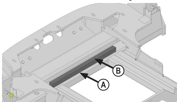
3. Clean top of undercarriage tube (A). Cut foam (B) to 37".
