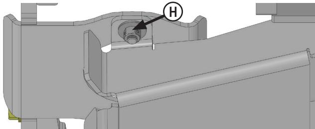
7. Attach bottom cover plate to rear clamp bracket with 2 - 1/2" flat washers, and 2 - 1/2" lock nuts (H).
