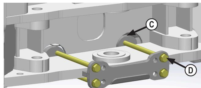
7. Lift undercarriage and push undercarriage back until vertical push plates (C) are firmly against cross member and all 4 holes are exposed.
